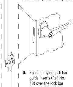
4. Slide the nylon lock bar guide inserts (Ref. No. 13) over the lock bar ends and through the door slots (see "B" at right). Push down firmly until the guides snap into place.
