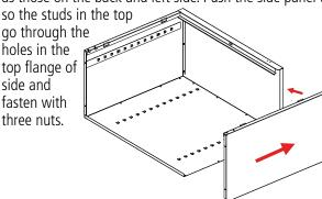
**6.** Attach the sill (Ref. No. 6) to the sides. Place nuts loosely on each of the studs and slide the ends of the sill into the slots on both sides of the unit. Then, securely tighten the nuts.
