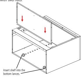
**8.** Set the unit upright and tighten all the nuts and bolts around the entire unit.
