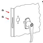
1. Place the locking handle (Ref. No. 11) on the right hand door and fasten with two #8-32 X 1/4 hex-head bolts and lock washers, provided with the handle.
