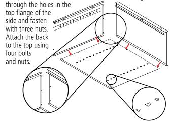
**5.** Attach the right side (Ref. No. 3) to the back in the same manner as you did in step 3, again making sure that the flange is around the back and that the lances on the shelf adjustment strips are pointed in the same direction as those on the back and left side. Push the side panel up
