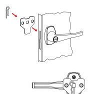
With the handle still in the open position, hook the locking bars (Ref. No. 10) to the locking cam (see "A" at left). Once in position, slowly rotate the door handle to the closed position so the lock bars prot rude from the holes at the top and bottom of the door (shown at right, below).
