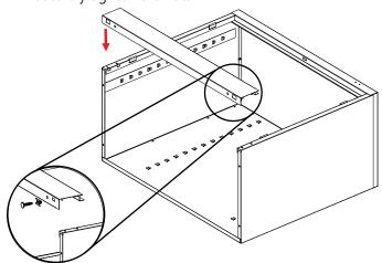
**7.** Place the rear flange of the bottom (Ref. No. 9) into the bottom lances of the back. The flange with two holes should face the front, hanging over the sill. Insert bolts through the bottom and sill with the head facing the front of the unit. Secure with two nuts.
