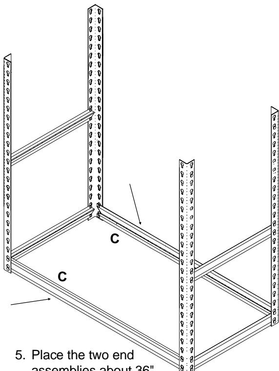
5. Place the two end assemblies about 36" apart, with the angled corners facing outward. Connect two 36" shelf supports (Ref. C) between the two assemblies, one on each side, as shown. Be sure to use the two keyhole slots nearest the floor, as before.
