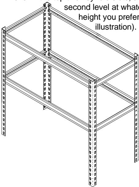
B. Instead of stacking the uprights on top of each other, as shown in step seven inside this sheet, place four shelf supports in the top two keyhole slots, being sure that the flat edge of each shelf support is facing up as described in earlier steps.
