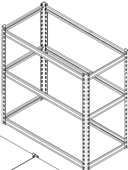
D. Insert one particleboard shelf at each of the five shelf levels, as described in step 11 inside this sheet. Then, place the two units together, or use separately as desired. Your Stur-D-Stor Shelving System is now ready for use.
