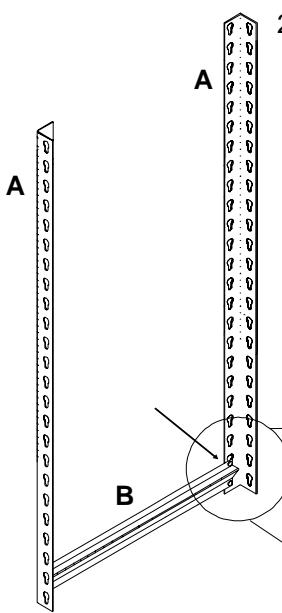
2. Connect two upright posts (Ref. A) with a 18" wide shelf support (Ref. B) by inserting shelf support rivets into the bottom two keyhole slots of each upright. Use a rubber mallet to seat the upright securely in the keyhole slots.
