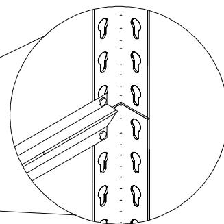
7. Mount another upright post (Ref. A) to the top of one of the other uprights and attach with an 18" shelf support, mounting the bottom rivet of the shelf support in the bottom upright post, and the top rivet in the new upright post, as shown in the exploded view above.
