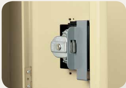
Master Gravity Lock Master Gravity Locks feature a built-in combination lock with an automatic locking lift handle and a vertically operating bolt to ensure security of contents.
